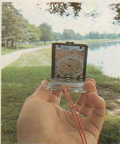
Map properly oriented with compass. Note the base plate is aligned with declination indicator. True north is signified by line and star to left of base plate. All USGS topographic maps are so marked.
